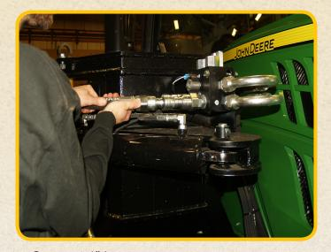
Connect 1" hoses. Wrap hoses in teflon wrap. Wrap is located in the cab of tractor.
