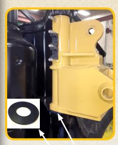
Thrust Washer goes under bottom of swivel.
