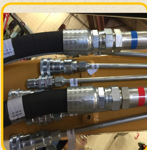
Attach all lines so that controls can be used to help lift and align boom arm with swivel pin.
