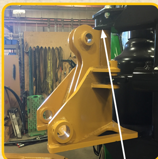
Lift boom Swivel with over head hoist and align with pin.
