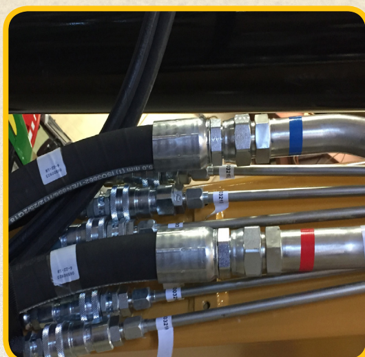
Connect lines to matching labeled male and female ends.
