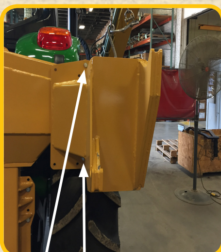
Take out 6 bolts in stow plate and slide to far right, this is the working position for stow.
