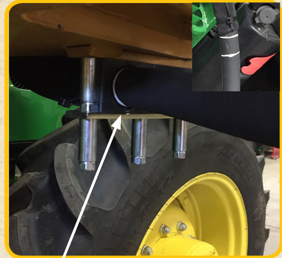
Attach 1" hose to clamp under swivel on top bracket. White line marks are 40" from end of 1" line to hose clamp. 1/4" lines go on bottom bracket.
