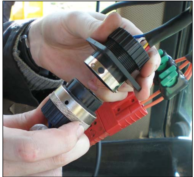
Connect control lines to the machines control unit in the tractor cab ( Electric models only ).
