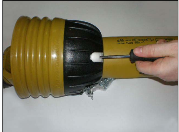
Insert screwdrivers into the clasps
