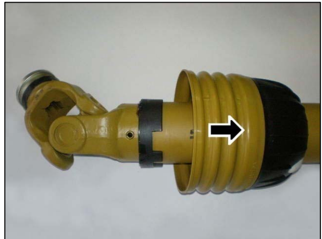
Slide shield back to reveal universal joint
