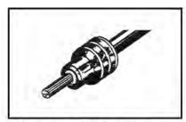
2. Align seal with cable insulation.
