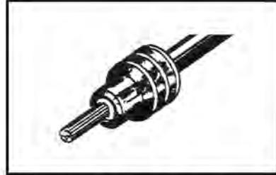
2. Align seal with cable insulation.
