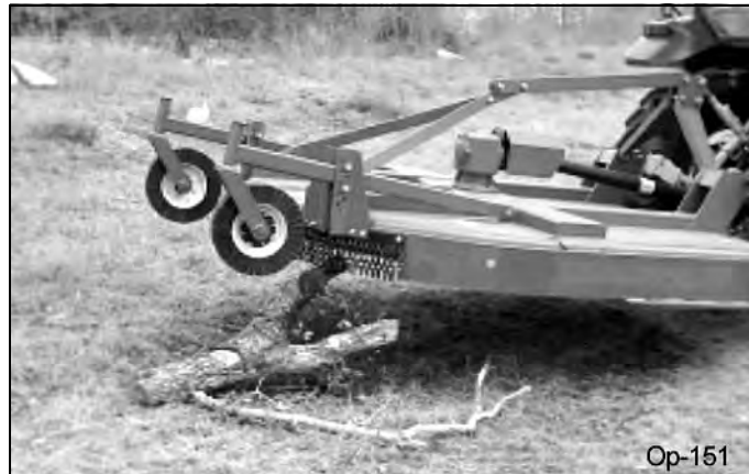
Raise Mower over solid objects
