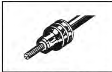
2. Align seal with cable insulation.
