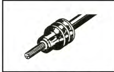
2. Align seal with cable insulation.
