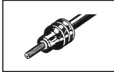
2. Align seal with cable insulation.
