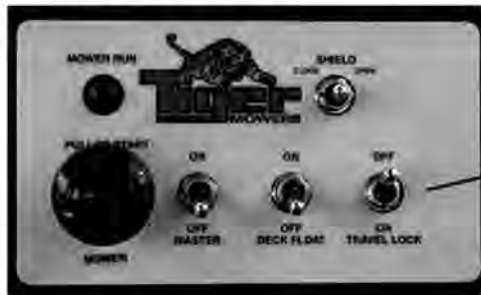
ELECTRONIC LIFT VALVE SWITCH BOX
