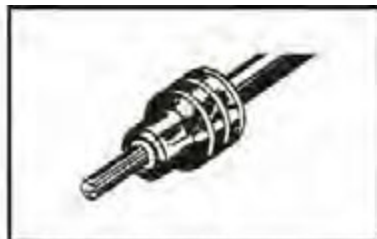
2. Align seal with cable insulation.
