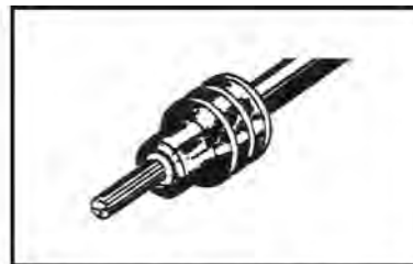
2. Align seal with cable insulation.
