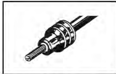
2. Align seal with cable insulation.
