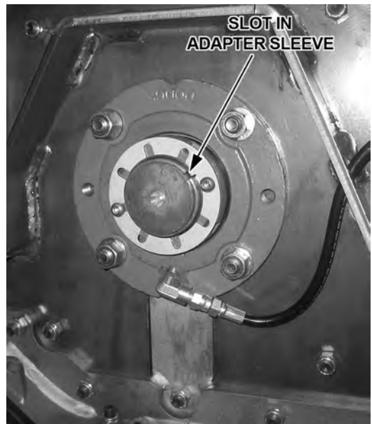
Install hardened washers, apply Loctite 271 to studs, and torque nuts to 61 ft.-lbs.
