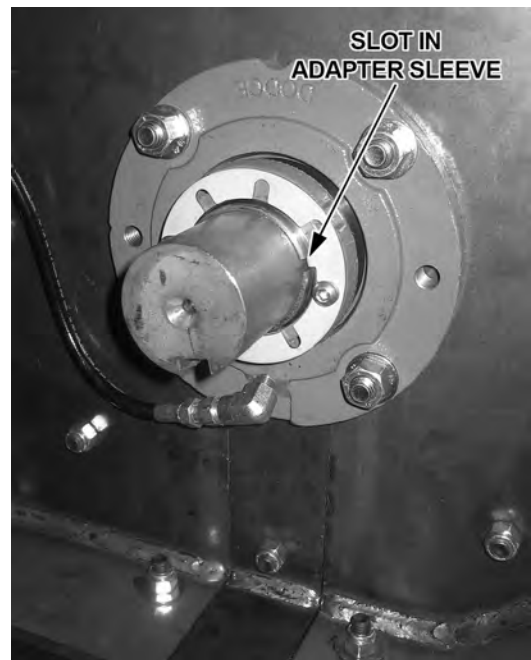
Install hardened washers, apply Loctite 271 to studs, and torque nuts to 61 ft-lbs.
