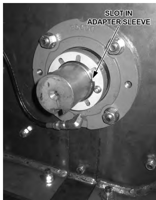
Install hardened washers, apply Loctite 271 to studs, and torque nuts to 61 ft-lbs.
