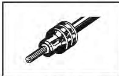
2. Align seal with cable insulation.
