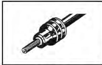
2. Align seal with cable insulation.
