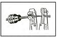
1. Apply seal to cable, before stripping insulation
