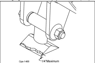
Failure to replace worn or damaged blades may lead to catastrophic failure of the blades and ejection of the broken part with tremendous force which may cause serious bodily injury or death.
