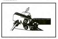
3. Put terminal in crimping tool, then position wire and seal in place.
