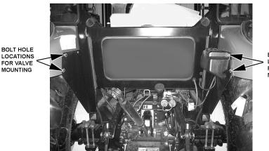
BOLT HOLE LOCATIONS FOR VALVE MOUNTING
