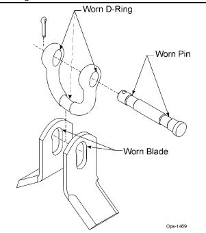
Always replace the pins and D-Rings whenever excessive wear is noticed.
