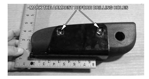
USE THE HARDWARE PROVIDED TO ATTACH THE BRACKET TO THE ARMEREST
