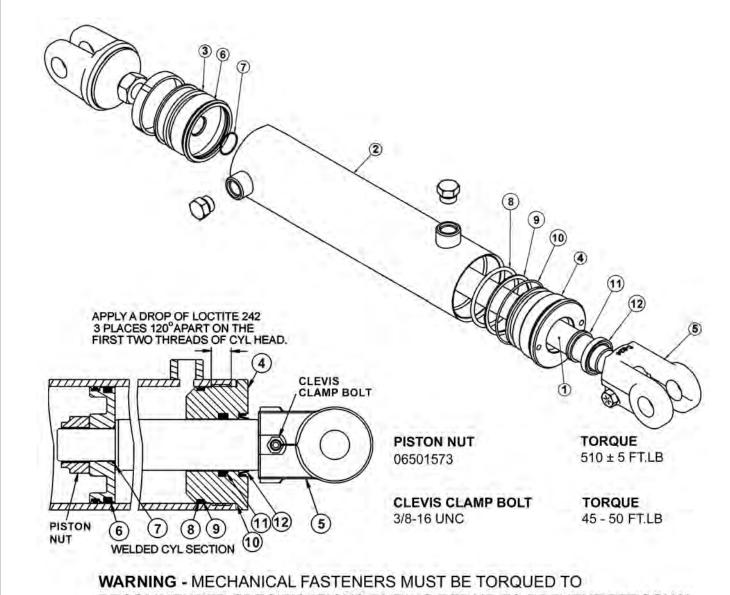
RECOMMENDED SPECIFICATIONS DURING REPAIR TO PREVENT PERSONAL INJURY OR EQUIPMENT DAMAGE.
