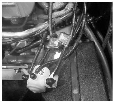
Route wires to and from the Continuous Duty Solenoid Switch as shown below.
