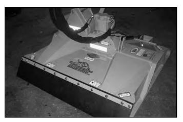
• Inspect the condition of deck skid shoes and hardware. OPS-B- 0025
