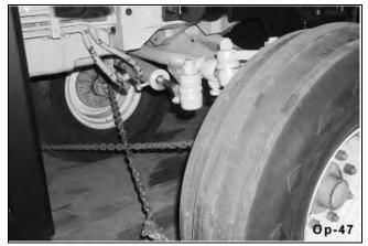
Arrange the chains so that when tightened, the chains are pulling downward and against themselves. Carefully tighten the securing chains or other fasteners using boomers or binders to apply maximum tension. Use extreme care when attaching and removing the securing devices as the extreme tension involved when released has the potential to inflict serious injury.
