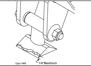
Failure to replace worn or damaged blades may lead to catastrophic failure of the blades and ejection of the broken part with tremendous force which may cause serious bodily injury or death.
