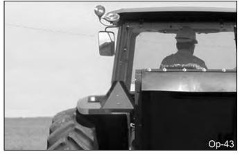
Make sure that all tractor flashing warning lights, headlights, and brake/taillights are functioning properly before proceeding onto public roads. While newer model tractors have plenty of lighting to provide warning signals and operating lighting, most older models where only equipped with operating lights. Consult an authorized tractor dealer for lighting kits and modifications available to upgrade the lighting on older tractor models. *OPS-B-0015*
