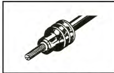
2. Align seal with cable insulation.
