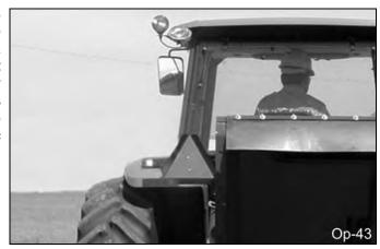
Make sure that all tractor flashing warning lights, headlights, and brake/tail lights are functioning properly before proceeding onto public roads. While newer model tractors have plenty of lighting to provide warning signals and operating lighting, most older models are only equipped with operating lights. Consult an authorized tractor dealer for lighting kits and modifications available to upgrade the lighting on older tractor models. *OPS-U-0021*
