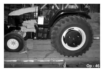
Use adequately sized and rated trailers and equipment to transport the tractor and implement. Consult an authorized dealer to determine the proper equipment required. Using adequately sized chains, heavy duty straps, cables and/or binders, securely tie down both the front and rear of the tractor utilizing the proper tie down locations as specified by the tractor manufacturer. *OPS-U- 0025*
