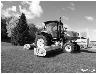
The mower must be operated with the cutter sections fully lowered and the hydraulic control lever in the float detent to ensure the mower follows the contour of the ground and to prevent sections from creeping up. NEVER attempt to raise the mower while the mower is operating.
