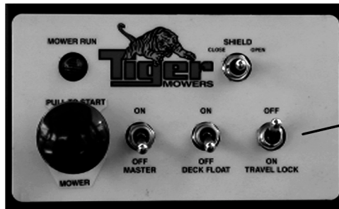
ELECTRONIC LIFT VALVE SWITCH BOX
