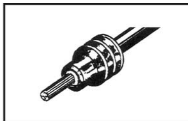
2. Align seal with cable insulation.
