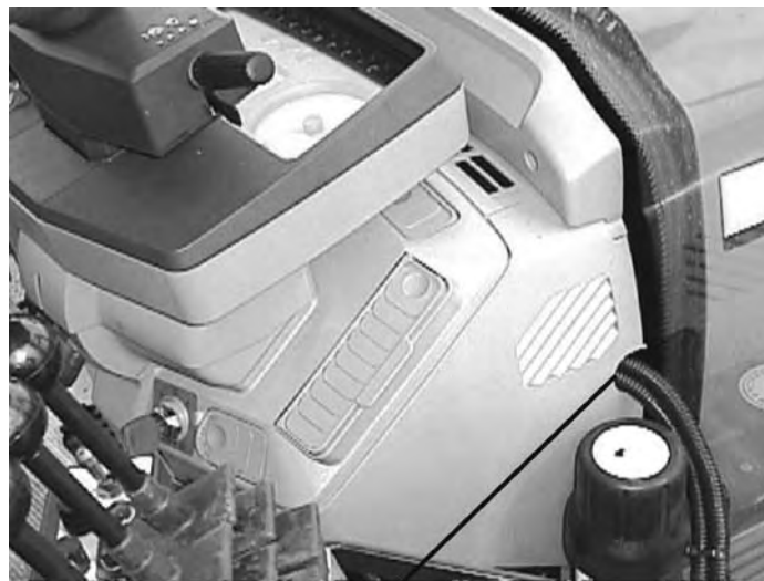
CUT SLOT IN PANEL FOR WIRES FROM SWITCH BOX TO ENTER STEERING COLUMN
