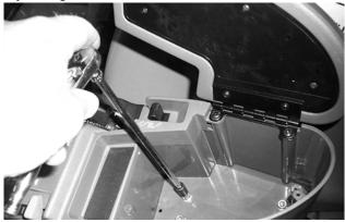
After removing the armrest, remove two screws from the IVT bracket/Slider assembly. You may have to adjust the slider assembly as shown below to obtain access to the screws.
