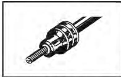
2. Align seal with cable insulation.
