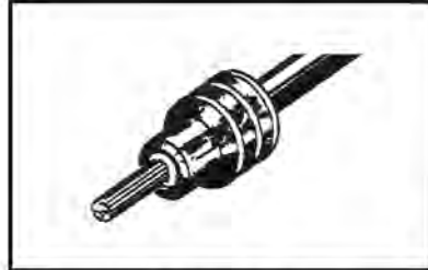
2. Align seal with cable insulation.
