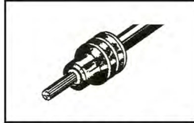
2. Align seal with cable insulation.
