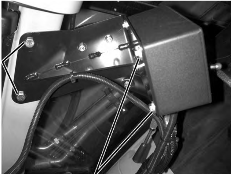
SWITCH BOX MOUNTING BOLTS
