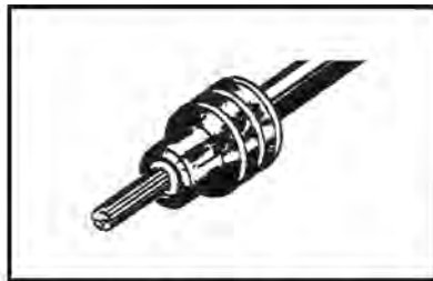
2. Align seal with cable insulation.
