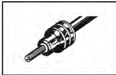
2. Align seal with cable insulation.
