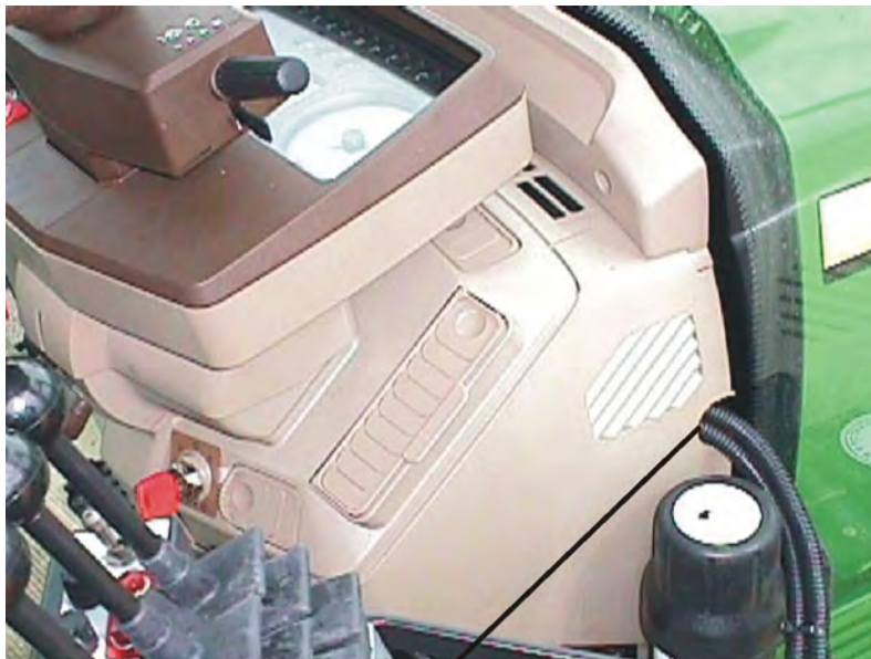
CUT SLOT IN PANEL FOR WIRES FROM SWITCH BOX TO ENTER STEERING COLUMN
