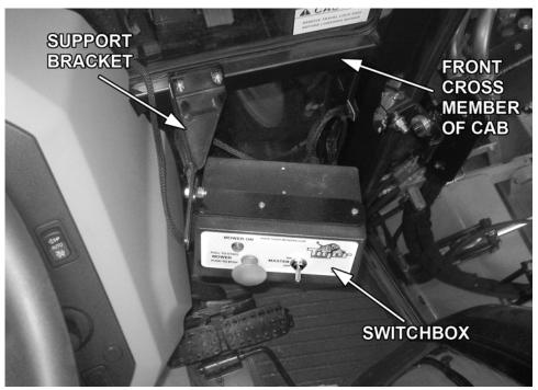
After installation of switchbox brackets 06411086, apply clear RTV (silicon) seal all around the outside of the bracket to prevent leaks. (ASM-JD-0087 Side JD5075E).
