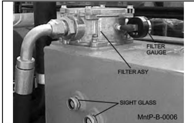
If your reservoir has one sight glass/temperature gage: The reservoir should be filled to the center of the sight glass on the side of the tank. Do not over-fill. If the tank has too much oil, the excess may be expelled through the pressurized breather.
