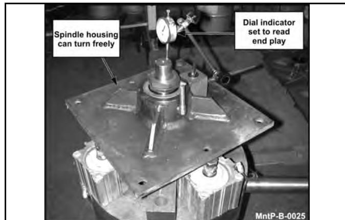
If the end play is correct, 0.001 inch to 0.003 inch, bend tabs up on jam washer to prevent the lock nut from loosening.
