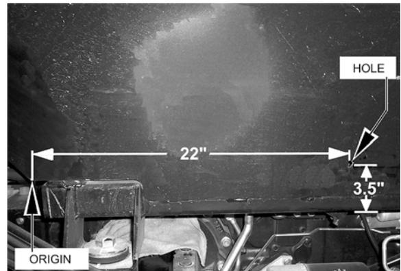
Place as many hoses in the clamp as will fit without compromising pressure. Then secure the (2) HOSE CLAMP (06520013) to the holes drilled with (1 EACH) CAPSCREW, 3/8 X 1 NC (21630) and (1 EACH) NYLOCK NUT, 3/8 NC (21627). The hoses that don't fit into the clamp are to be secured to the others with zip ties. For protection of hoses in contact with metal edges, wrap hoses with split hose sections and fasten with hose clamps or zip ties as needed.
