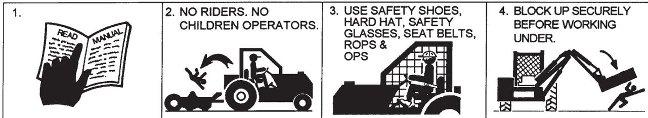
1. Study and understand Operator's Manuals, Safety Decals, and Instructional Decals for tractor and implement to prevent misuse, abuse, and accidents. Practice before operating in a confined area or near passersby.
