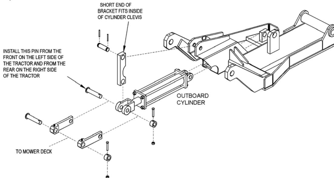
Slide other end of pivot arm with short distance between the cutout and the end of the pivot arm, into the cylinder clevis. Next, line up the holes of the left and right lift linkage arms outside of the cylinder clevis holes. Connect with linkage pin, shims (as required), boss, capscrew, lockwasher and hex nut as shown.
