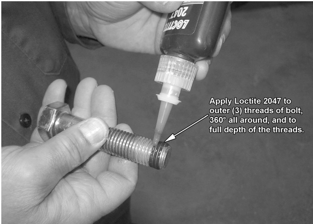
Apply Loctite 2047 to outer (3) threads of bolt, 360° all around, and to full depth of the threads.
