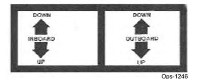
The rear mower height is controlled with the 3-point hitch control lever. Follow the instructions for this control in the tractor operator's manual. The tilt of the rear mower is controlled with the third spool of the lift valve, and is coordinated as shown in **Figure Ops-1246.**
