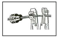
Apply seal to cable, before stripping insulation.
