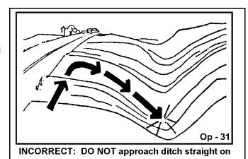
Inclines and ditches should be approached along a line which is at an angle as shown. This type of path will reduce the possibility of resulting damage. If the gradient is so steep that such an approach increases the possibility of a tractor roll-over, select an alternate crossing path.
