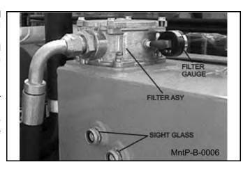
If your reservoir has one sight glass/temperature gage: The reservoir should be filled to the center of the sight glass on the side of the tank. Do not over-fill. If the tank has too much oil, the excess may be expelled through the pressurized breather
