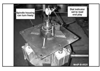
5. After the lock nut is tightened, there must be 0.001 inch to 0.003 inch of free play when lightly prying up on the spindle housing.
