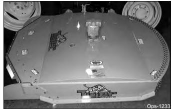
Inspect the condition of deck skid shoes and hardware. OPS-R-216
