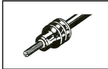
2. Align seal with cable insulation.
