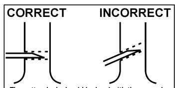
The cutter deck should be level with the ground to reduce the work required by the cutter and tractor to minimize equipment wear and damage.
