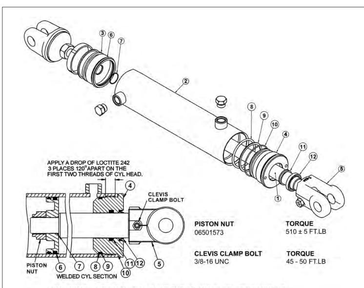
**WARNING -** MECHANICAL FASTENERS MUST BE TORQUED TO RECOMMENDED SPECIFICATIONS DURING REPAIR TO PREVENT PERSONAL INJURY OR EQUIPMENT DAMAGE.
