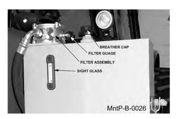
The reservior should be filled to the center of the sight glass on the side of the tank. Do not over-fill. If the tank has too much oil, the excess may be expelled through the pressurized breather.
