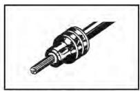
2. Align seal with cable insulation.
