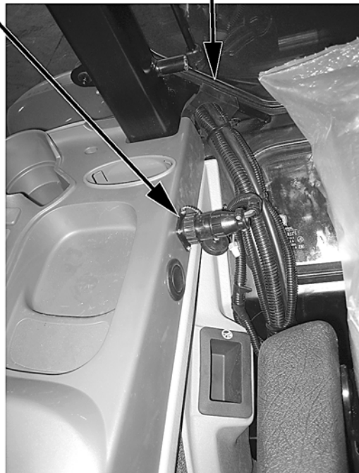
REAR WINDOW WITH RUBBER GROMMET
