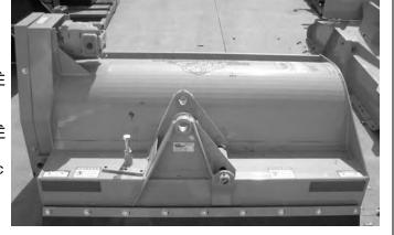
The cutter deck should be level with the ground
