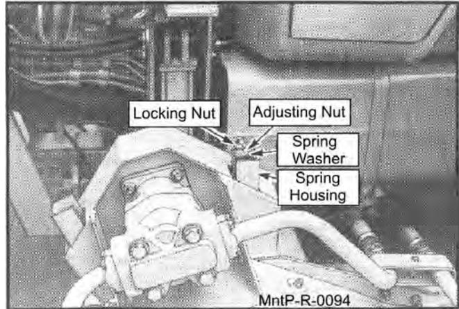
For standard cut on the mechanically driven rear flail mower, adjust so that the spring washer is flush with the spring guide. **MntP-R-0095**
