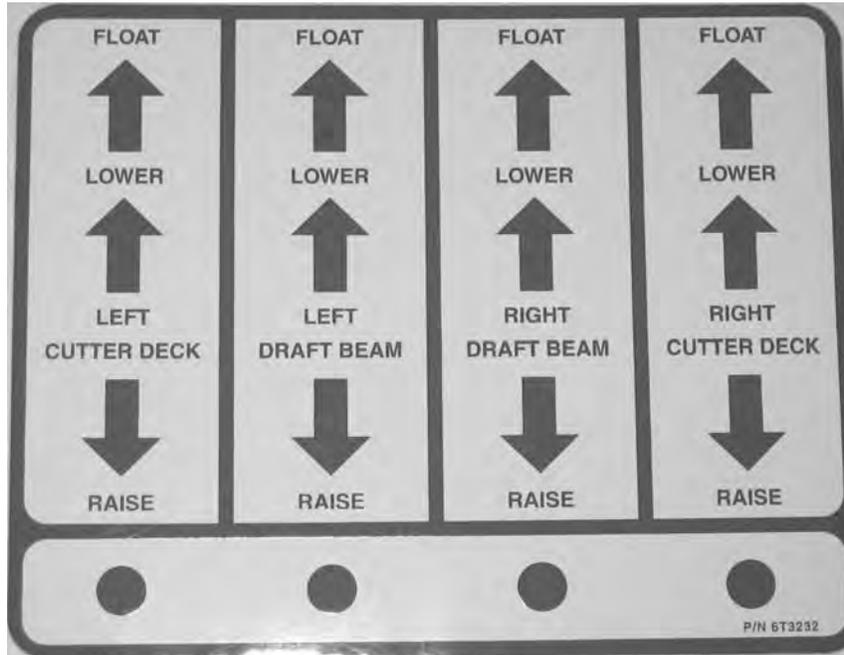
The rear mower height is controlled with the 3-point hitch control lever. Follow the instructions for this control in the tractor operator's manual. The tilt of the rear mower is controlled with the third spool in the lift valve and is coordinated as shown above.
