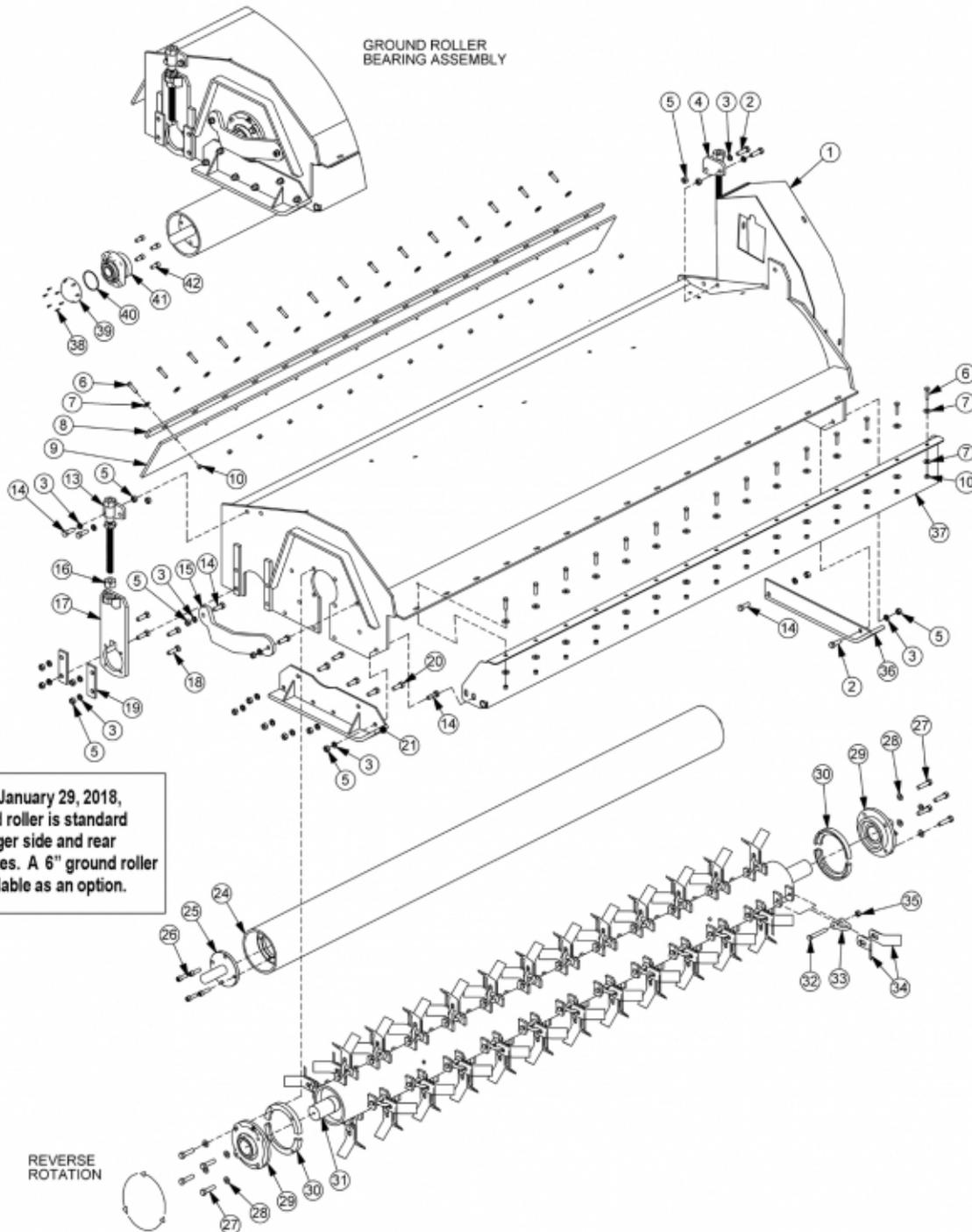
NOTE: As of January 29, 2018, an 8" ground roller is standard on all new Tiger side and rear flail assemblies. A 6" ground roller remains available as an option.
