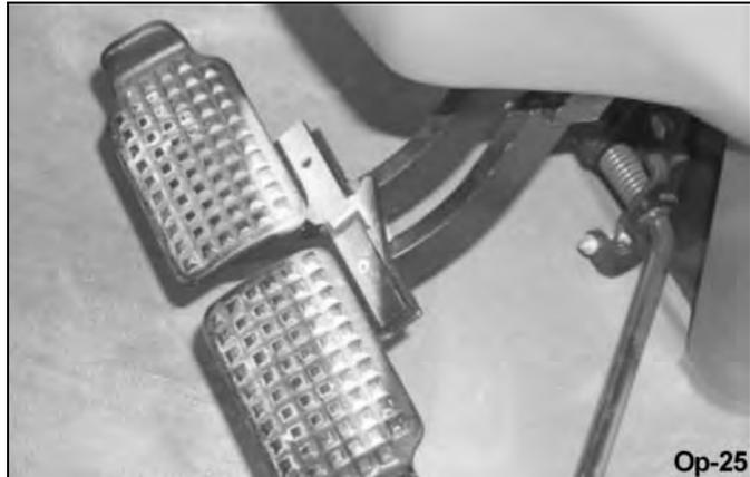
Use extreme caution and avoid hard applications of the tractor brakes when carrying equipment at road speeds. Never haul the implement at speeds greater than 20 MPH (32 kph). OPS-U- 0018\_A
