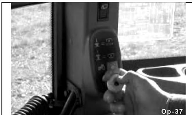
Park the tractor on a level surface, place the transmission in park or neutral and apply the parking brake, lower the attached implement to the ground, shut down the engine, remove the key, and wait for all motion to come to a complete stop before exiting the tractor. OPS-F-0011
