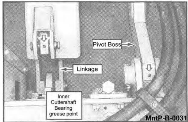
With the cutter head lowered, locate the grease zerks on the linkage and pivot bosses. Inject Lithium-Complex Extreme Pressure grease conforming to NLGI2-ISO 320 specifications until it protrudes from the ends. With the cutter head in this position, it is also possible to grease the draft beam cylinder anchors and pins. Now, raise the cutter head to expose the remaining zerks on the deck tilt linkages and on the other end of the cylinder.
