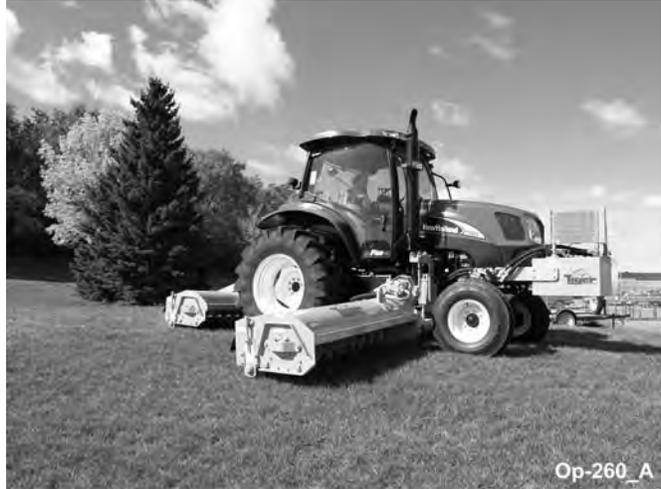
The mower must be operated with the cutter sections fully lowered and the hydraulic control lever in the float detent to ensure the mower follows the contour of the ground and to prevent sections from creeping up. NEVER attempt to raise the mower while the mower is operating.
