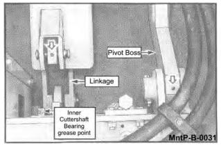
With the cutter head lowered, locate the grease zerks on the linkage and pivot bosses. Inject Lithium-Complex Extreme Pressure grease conforming to NLG12-ISO 320 specifications until it protrudes from the ends. With the cutter head in this position, it is also possible to grease the draft beam cylinder anchors and pins. Now, raise the cutter head to expose the remaining zerks on the deck tilt linkages and on the other end of the cylinder.
