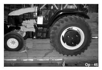
Use adequately sized and rated trailers and equipment to transport the tractor and implement. Consult an authorized dealer to determine the proper equipment required. Using adequately sized chains, heavy duty straps, cables and/or binders, securely tie down both the front and rear of the tractor utilizing the proper tie down locations as specified by the tractor manufacturer. *OPS-U- 0025*
