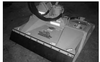
Inspect the condition of deck skid shoes and hardware. OPS-B- 0025
