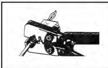
3. Put terminal in crimping tool, then position wire and seal in place.
