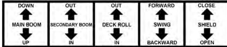
Diagram illustrating the control panel layout and the corresponding hydraulic lines for the CD9F5HCB. The panel includes controls for the Main Boom, Secondary Boom, Deck Roll, Swing, and Shield. The hydraulic lines are labeled with their respective functions: Pressure & Return, Main Boom, Secondary Boom, Deck Roll, Boom Swivel, Safety Shield, and Load Sense.
