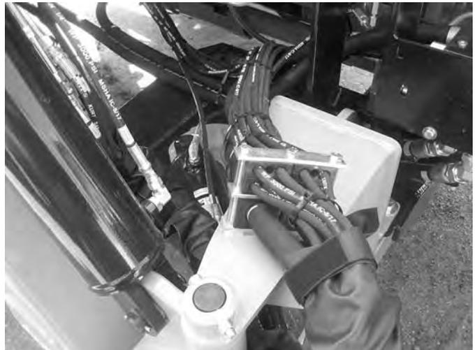
The rear stow Bengal hose routing is only for machines with a front-mounted PTO. If you have a rear-mounted PTO, you must use the front stow Bengal hose routing. For more information, see the front stow Bengal hose routing section of this manual. The rear stow Bengal hose routing is only for machines with a front-mounted PTO. If you have a rear-mounted PTO, you must use the front stow Bengal hose routing. For more information, see the front stow Bengal hose routing section of this manual.
