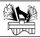
Tank contents under pressure. Allow oil to cool before slowly removing cap
