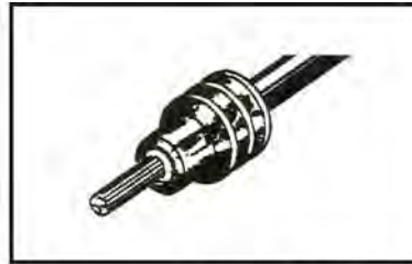
2. Align seal with cable insulation.
