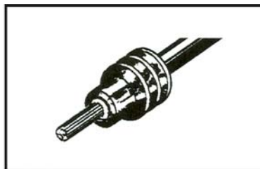
2. Align seal with cable insulation.
