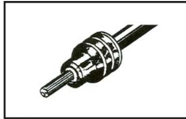
2. Align seal with cable insulation.
