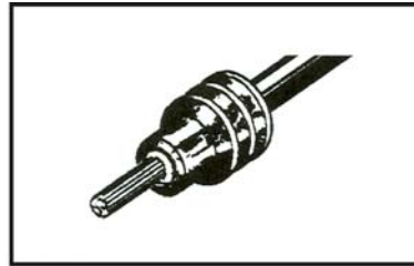
2. Align seal with cable insulation.
