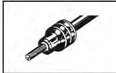
2. Align seal with cable insulation.
