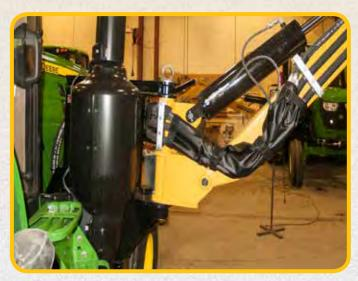
Connection complete - back side view. **Approx.** 4 hrs shop time to complete assembly.
