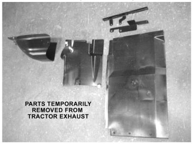
When removing heat shield parts from the tractor exhaust, save all hardware to re-install the heat shield after the John Deere tube bracket has been replaced
