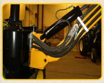
Run 1" lines on bottom 2 spaces of clamp and run 1/4" lines on top space. Measurement is 38" for 1" lines, clamp to clamp. Match 1/4".
