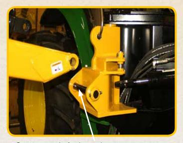
Connect end of primary boom arm to swivel with horizontal pin.
